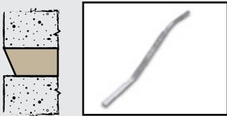
**V-Joint** This type of joint is made with the help of a curved steel tool with a 'v' shaped end. Proper tooling of the v-joint helps to prevent water accumulation in the joint.
