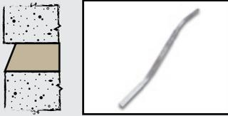
**Struck Mortar Joint** The bottom edge is recessed while the top edge will be finished flat with the brick edge. The slope provided here will pull water and hold it in the brick, so it is best suited for interior walls only.
